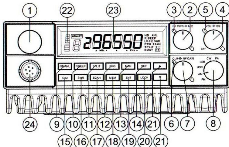
1. **FREQUENCY SELECTOR:** Used to set the desired transmit and receive frequency. The frequency is digitally displayed in the LCD window next to the selector. The FREQUENCY SELECTOR knob next to the LCD display, allows changing each digit on the frequency display by first placing the frequency display cursor (using SHF button) below the desired digit and then turning the selector knob.
