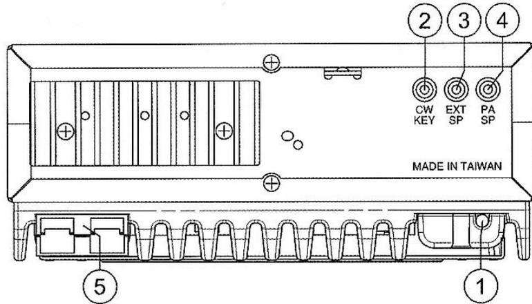
1. **ANTENNA:** This jack accepts a 50 ohms coaxial cable with a PL-259 style plug.
