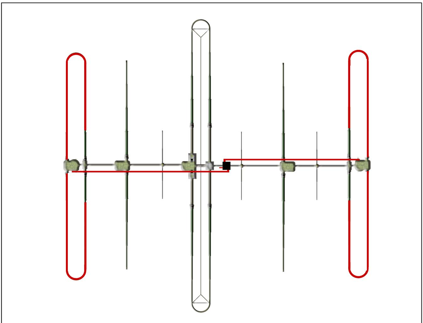
The 80m dipole option is a wire dipole that runs above and parallel to the boom. One end of the wire dipole connects to the reflector element center, the other end connects to director 2. This forms an "H" shaped dipole, as shown below in figure X.
